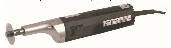
**30.216.22** Oscillating cast cutter 500 W "heavy duty", 230 V~, 50/60Hz and 500 Watt, with variable control of oscillations, very silent motor with an ergonomic housing, can be used for big and even thick walled bandages such as bandages for the thoracic and pelvic area.
