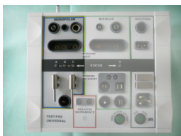
Testing area for monopolar cords, electrode pens/handles
