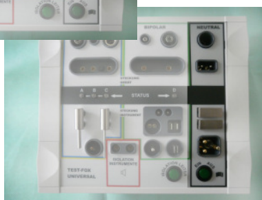
Testing area for cables for neutral electrodes
